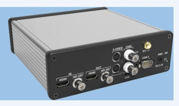
The Proteus is a high-performance stand-alone High-Definition (HD) and Standard-Definition (SD) video overlay system. It overlays crisp text, graphics and telemetry data on live video. From overlaying GPS informations and custom titles to more advanced graphic widgets, users can easily customize Proteus with external keyboard or simple RS232 commands.
